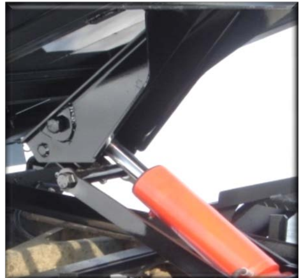
Compact, yet rugged scissor hoist with a 6,000 lb. lift capacity
